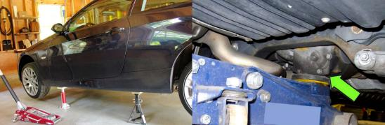
Step 1- You will need to lift your car up to access the drain plug. I prefer to drive up on ramps and then level the car out by lifting the rear and placing the rear of the car on jack stands. Depending on what car you are driving, your rear center jack point will be somewhere on or near the differential or rear subframe. Don't lift the rear by the differential cover, especially if it is a finned cover. You will have to find out where the specific rear jack location is
